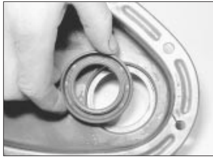
9.3 Timing cover oil seal must be fitted with the open side towards the chain
