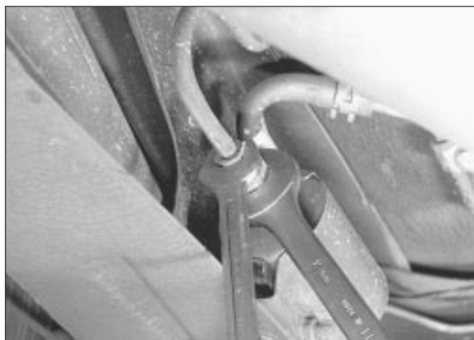
37.5b Slacken the union nuts whilst retaining the union adapter/filter with an open-ended spanner
