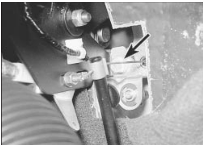
13.48 . . . then undo the retaining bolt (arrowed) and remove the accelerator pedal switch assembly from the car
