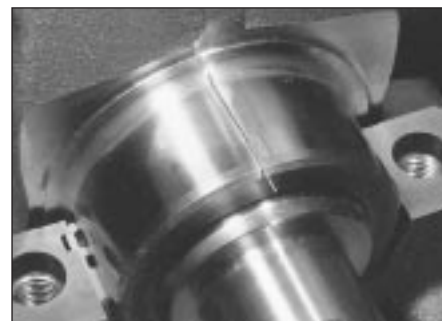
17.7 Plastigage in place on main bearing journal
