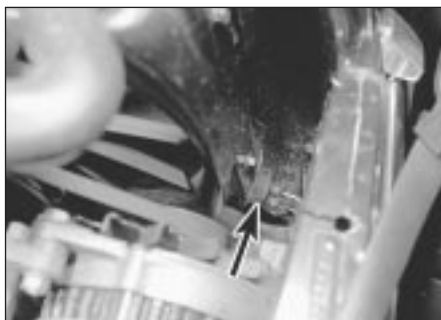
8.3 Auxiliary cooling fan switch location (arrowed) - fuel injection models
