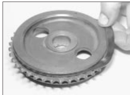
5.19 Fitting a new tensioning ring to the camshaft
