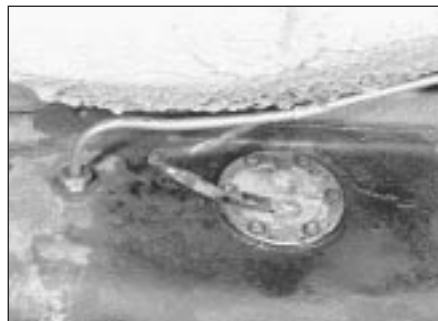
9.15 Fuel tank outlet pipe and fuel gauge sender unit (Estate, Van and Pick-up models)
