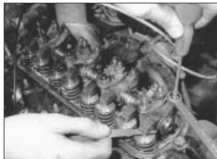
4.5 Adjusting the valve clearances
