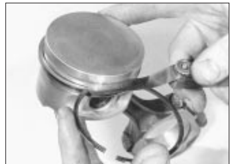
11.17 Measuring the piston ring-to-groove clearance
