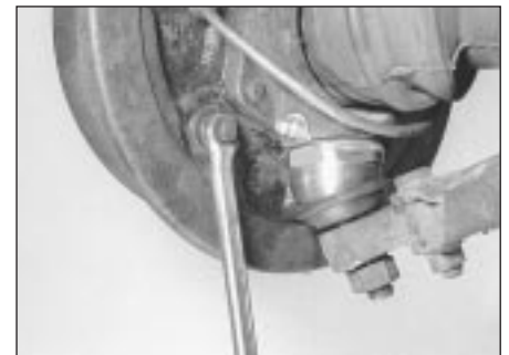
3.5 Adjusting one of the front brake adjusters with a brake adjusting spanner
