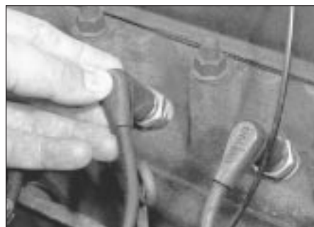
33.5 Pull the leads off the spark plugs by gripping the rubber boot
