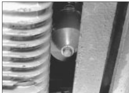
13.7 Cartridge type oil filter and retaining bolt as seen from below
