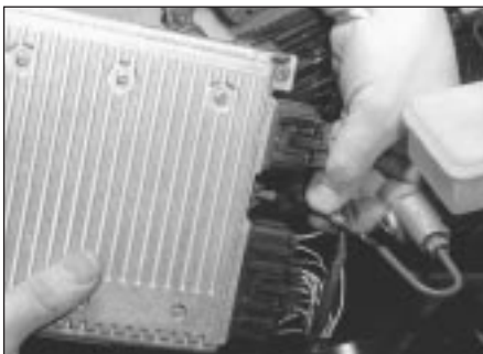
13.31 . . . then withdraw the ECU and disconnect the vacuum hose and wiring connectors
