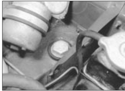
8.6 Subframe tower mounting bolt fitted to later models
