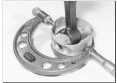
11.16 Measuring the piston diameter
