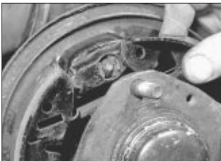
5.7a Withdraw the rear brake shoes from the brake adjuster pivots, detach the return spring . . .
