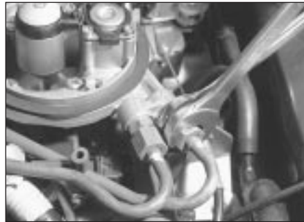
13.3 Retain the adapters with an open-ended spanner whilst slackening the fuel pipe union nuts
