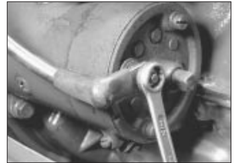
13.4a Unscrew the nut securing the starter motor cable
