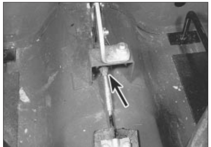
4.5b Handbrake cable adjusting nut on models with a single front cable
