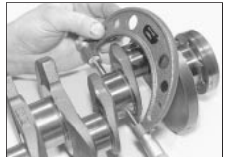
12.17 Use a micrometer to measure the crankshaft bearing journal diameters
