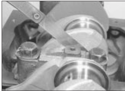
12.3 Checking crankshaft endfloat using feeler blades
