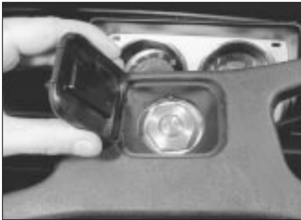
22.1 Prise up the central motif for access to the steering wheel nut on later models
