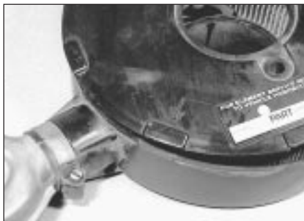
30.8 Make sure the alignment arrow is toward the lug on the air cleaner body
