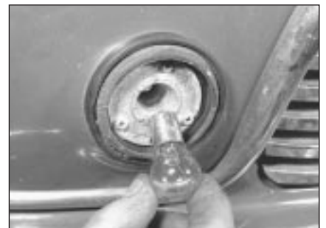
5.28 Push and turn the bulb anti-clockwise to remove
