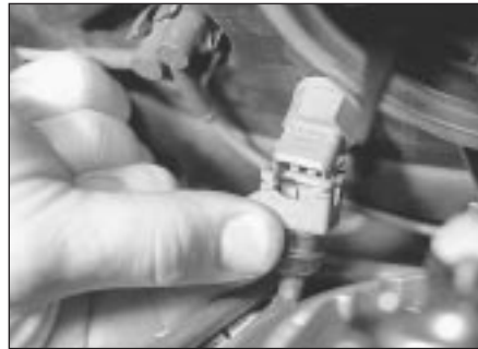
2.2a . . . then lift up the air cleaner assembly, and disconnect the intake air temperature sensor wiring connector . . .
