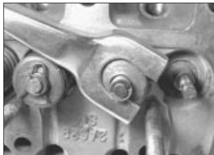
8.4a Compress the valve springs with a spring compressor and lift off the split collets . . .
