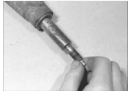
19.12c . . . then slide out the pivot shaft
