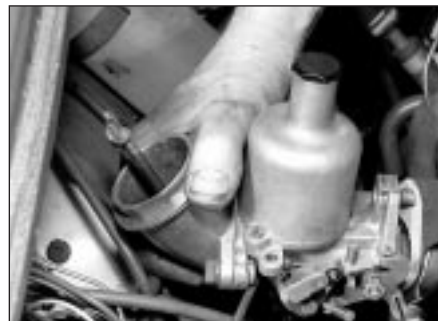
12.9 Removing the SU HS2 carburettor from the manifold
