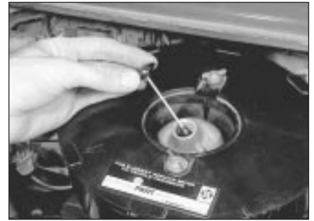
19.4 Top up the piston damper on carburettor models
