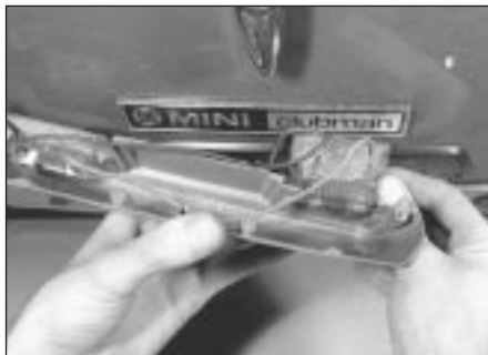
5.44 Removal of the number plate lens and bulb holder on Saloon models
