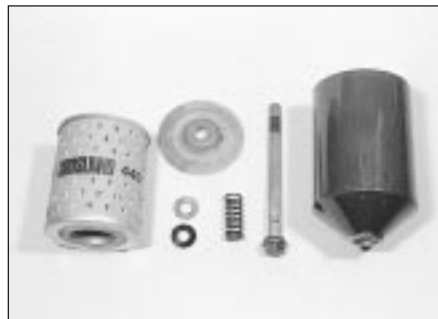
13.9 Components of the cartridge type oil filter
