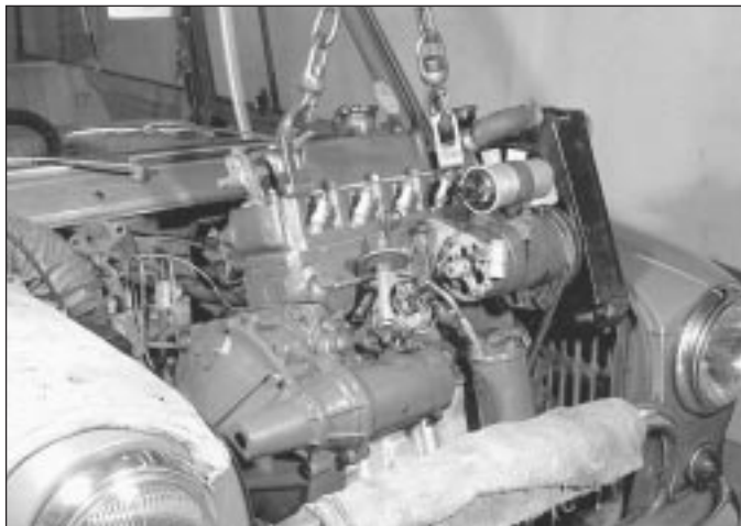
3.44a Lift the engine/transmission out of the engine bay . . .
