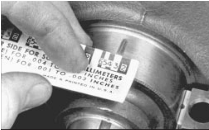
17.11 Measuring the width of the deformed Plastigage using the card gauge supplied
