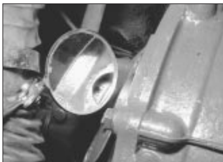
8.5 The timing marks on the flywheel can be viewed through the aperture in the housing using a mirror
