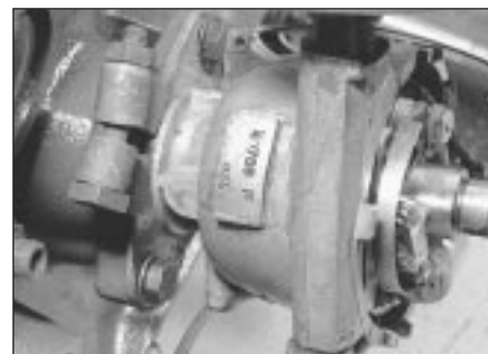
13.6 The distributor number is stamped on the body below the vacuum unit
