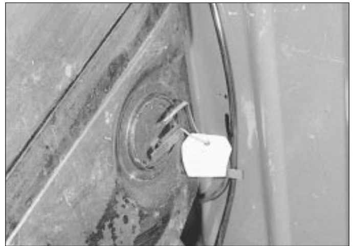
8.1 Electrical leads at the fuel gauge sender unit on the side of the tank (Saloon models)
