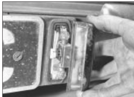
5.47 On Estate, Van and Pick-up models lift off the cover and lens . . .
