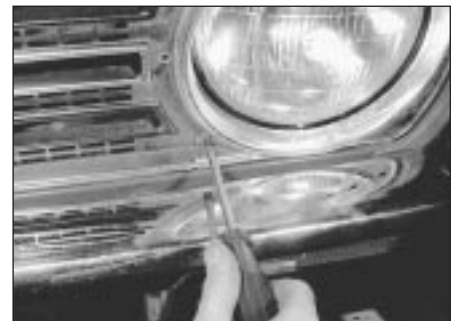
5.2a On Clubman models remove the grille panel extension for access to the headlight
