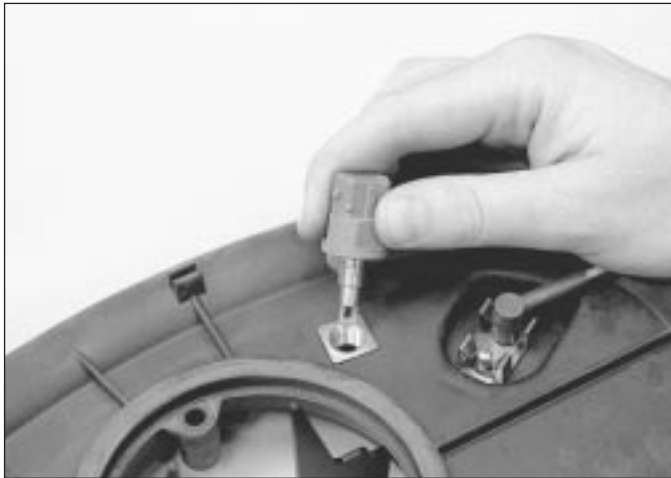
13.40 Removing the intake air temperature sensor from the air cleaner housing
