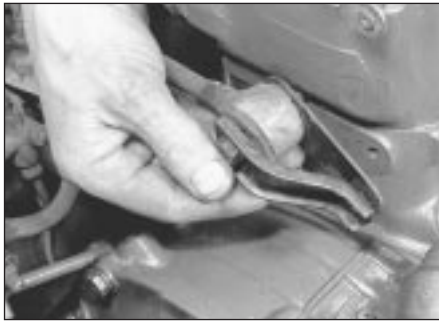
12.25 Removing the engine upper tie-bar from the cylinder block
