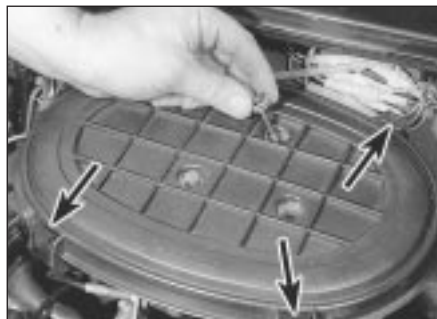
30.13a On fuel injection models, release the clips (three arrowed) and remove the screws
