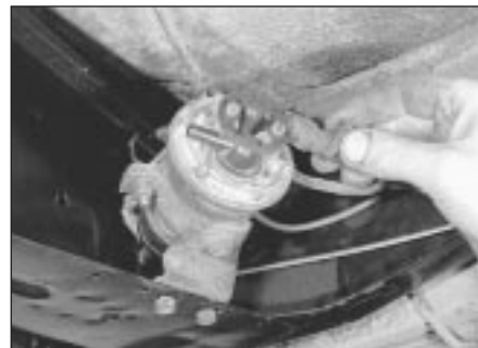
6.8 Removing the fuel outlet pipe from the electric pump
