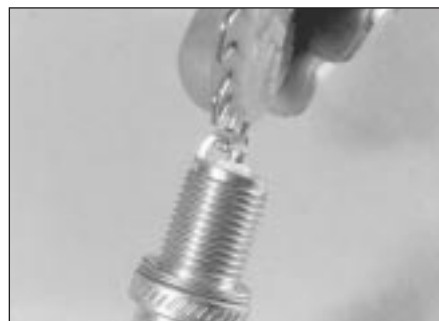
33.11 Adjusting a spark plug electrode gap
