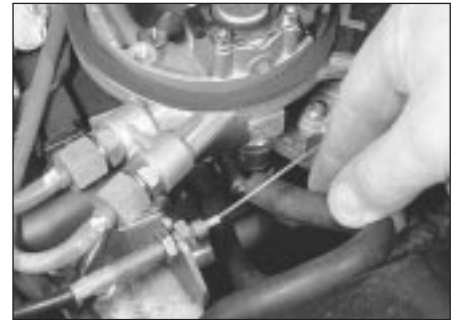
13.6 Disconnect the breather and purge valve hoses from the front of the throttle body assembly
