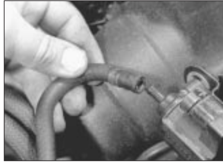
6.29 Release the retaining clip, and disconnect the outlet hose from the purge valve
